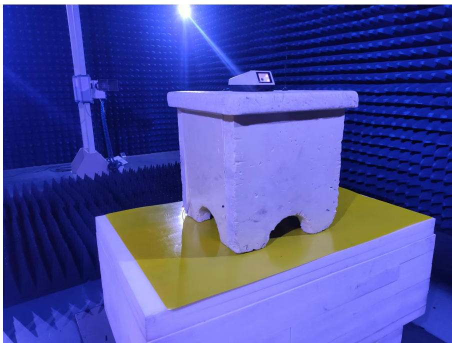
Photo of Radiated Emission Measurement (Above 1G)
