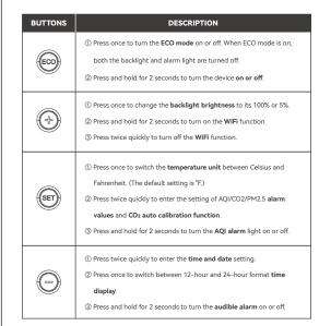
Note: When the device is powered off, place it in a well-ventilated place, then press and hold both the ECO and SET buttons simultan -eously, the device will enter the CO2 calibration mode. which takes 200 seconds. During the CO<sub>2</sub> calibration, please make sure that no one comes near the device to affect the calibration result.
