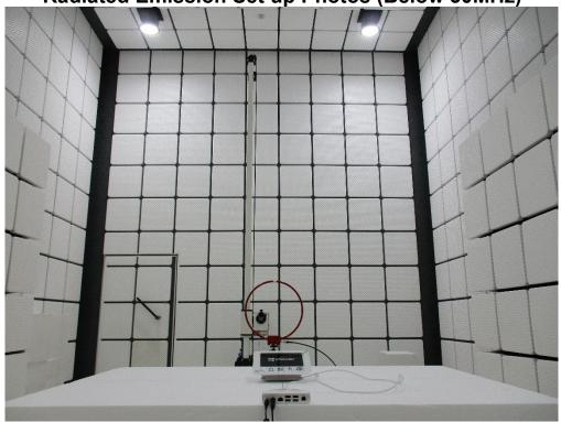
Radiated Emission Set up Photos (Below 1GHz)
