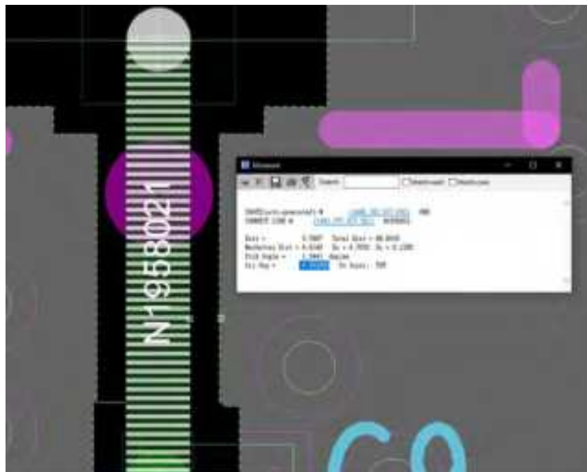
c. Air gap between RF trace and ground about 4.5 mil
