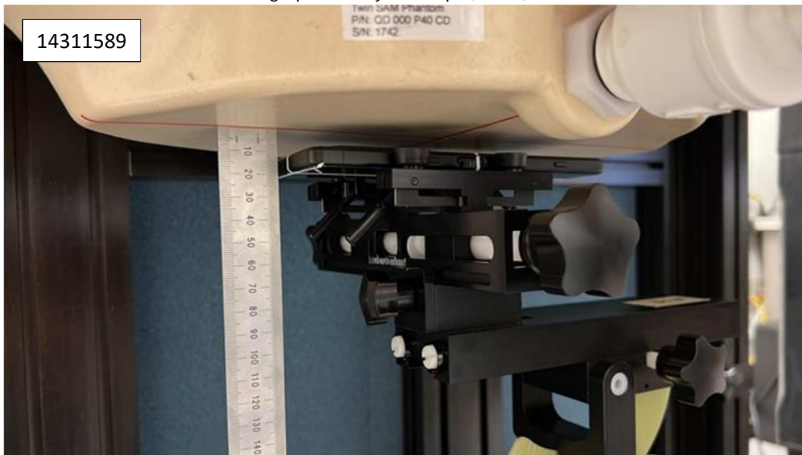
Photograph 9: Body & Hotspot, Rear, 10 mm
