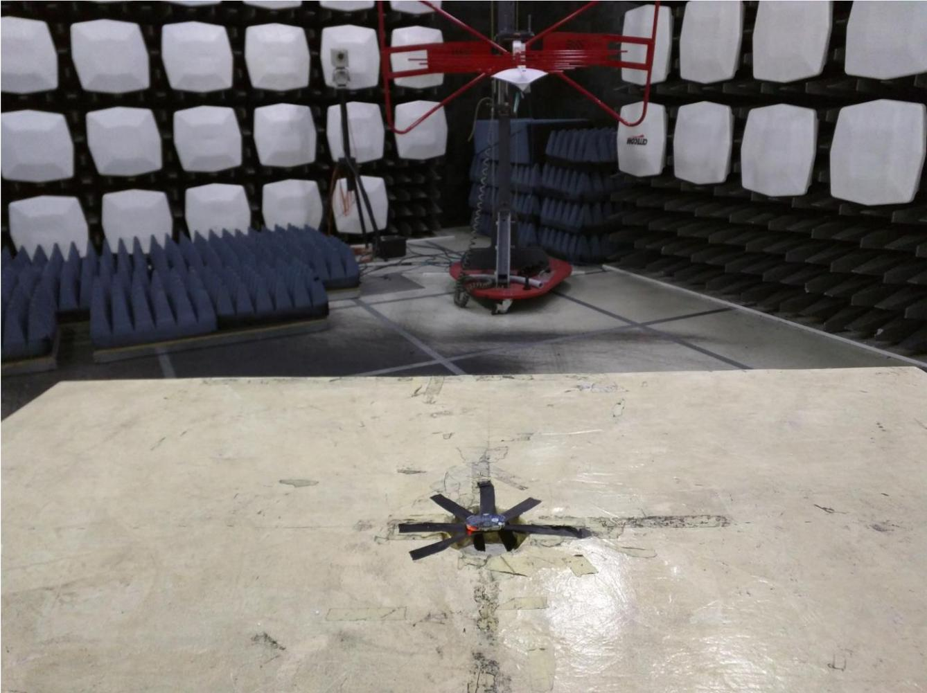
8. Radiated Emissions 1GHz- 3GHz Measurement
