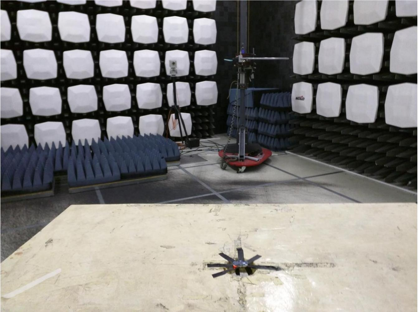
4 Radiated Emissions 30MHz- 1GHz Measurement
