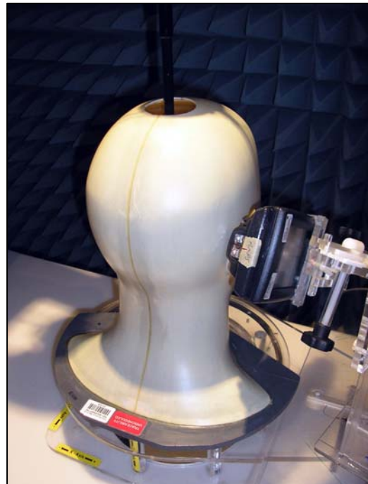
Figure 62. Positional photograph of the Intermec 700C Right Hand Cheek 15° Position
