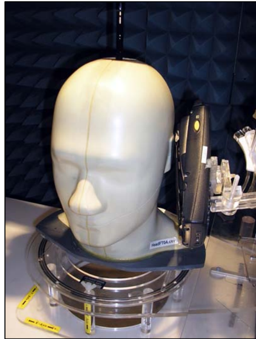
Figure 60. Positional photograph of the Intermec 700C Left Hand Cheek 15° Position
