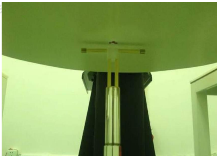
Photo of Dipole Setup
