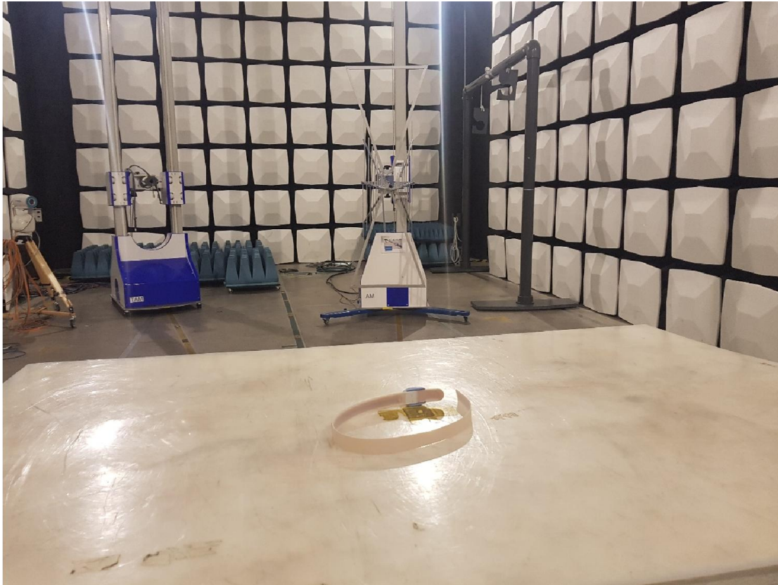
Test set up radiated emission 30 MHz – 1GHz
