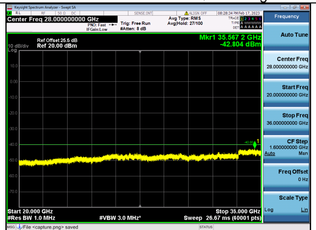
Band42C(3550~3600)-20G-36G / 20MHz+20MHz / 100RB+100RB/ QPSK / High CH
