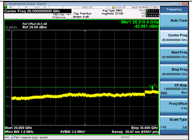
Band42C(3550~3600)-20G-36G / 20MHz+20MHz / 1RB+1RB/ QPSK / High CH
