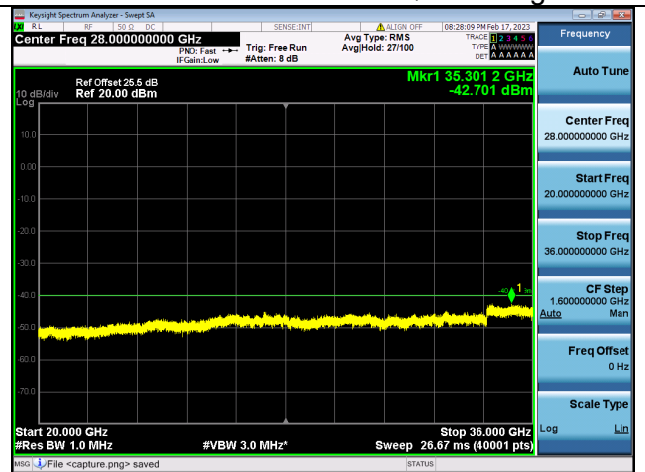
Band42C(3550~3600)-20G-36G / 20MHz+20MHz / 1RB+1RB/ QPSK / High CH
