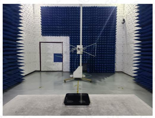
RADIATED EMISSION TEST SETUP ABOVE 1GHz
