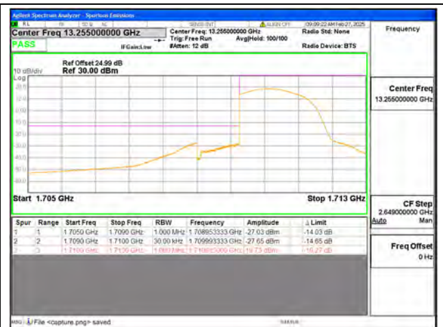
B4 / 1.4MHz / Low CH / QPSK / FULL RB
