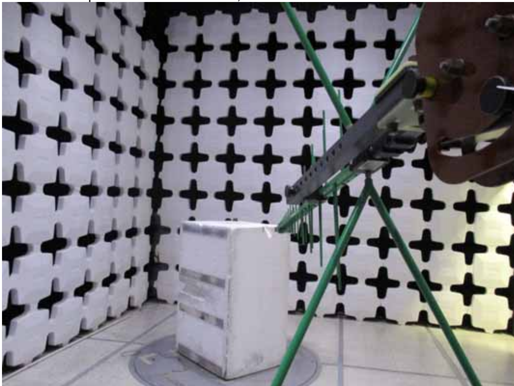
Test Setup for Radiated Emissions, 25MHz to 1GHz – Vertical Polarization
