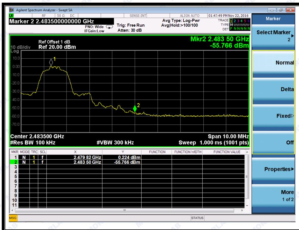
(Channel = 78, Band edge @ $\pi/4$ -DQPSK)
