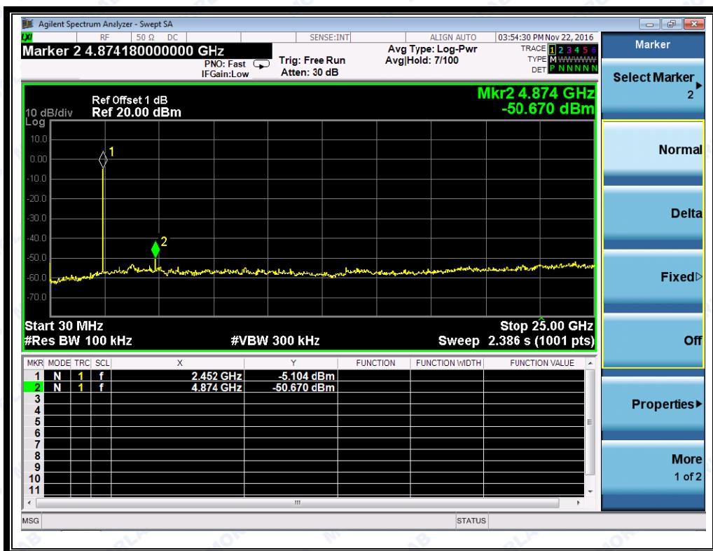
(Plot H.1: Channel = 39, 30MHz to 25GHz @ 8-DPSK)
