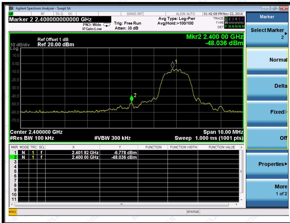
(Channel = 0, Band edge @ $\pi/4$ -DQPSK)
