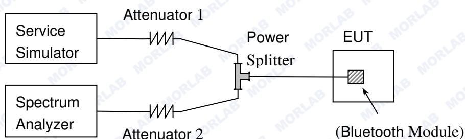
The Bluetooth Module of the EUT is coupled to the Spectrum Analyzer (SA) and the Bluetooth Service Simulator (SS) with Attenuators through the Power Splitter; the RF load attached to the EUT antenna terminal is 50Ohm; the path loss as the factor is calibrated to correct the reading. During the measurement, the Bluetooth Module of the EUT is activated and controlled by the SS, and is set to operate under test mode transmitting 339 bytes DH5 packages at maximum power.
