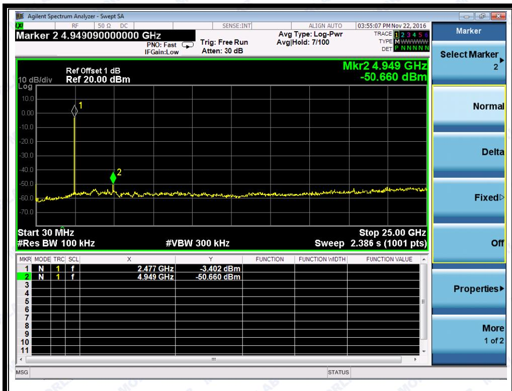
(Plot I.1: Channel = 78, 30MHz to 25GHz @ 8-DPSK)
