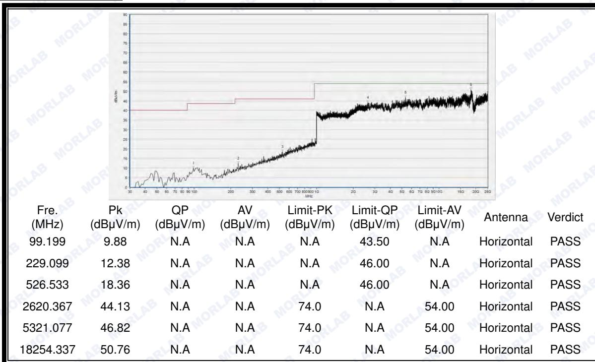
(30MHz to 25GHz, Antenna Horizontal @ GFSK, channel 0)
