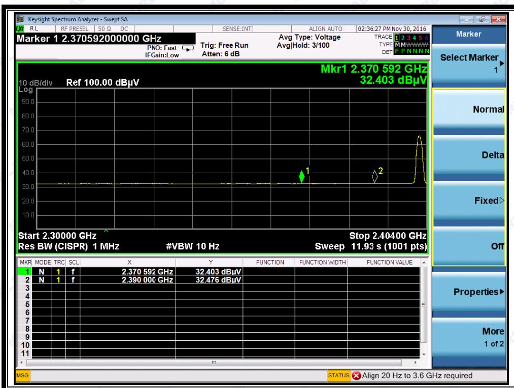
(Plot C2: Channel = 0 AVERAGE @  $\pi/4$ -DQPSK)
