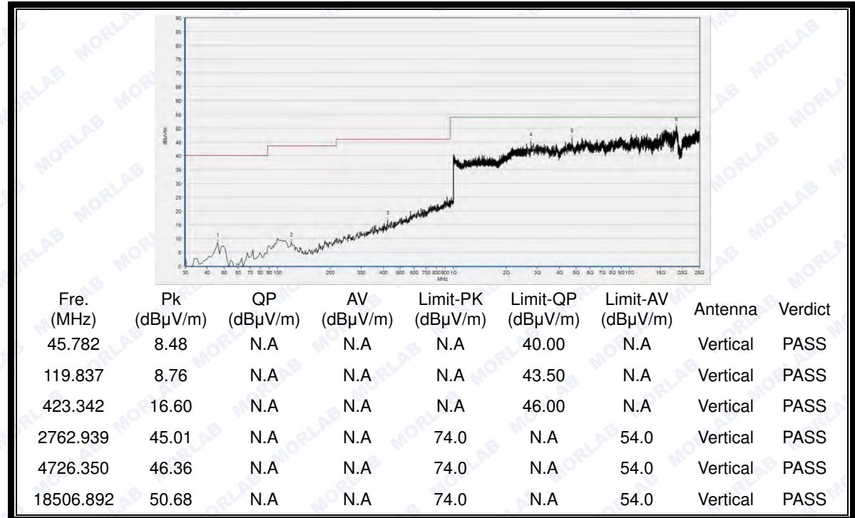
(30MHz to 25GHz, Antenna Vertical @8-DPSK, channel 78)
