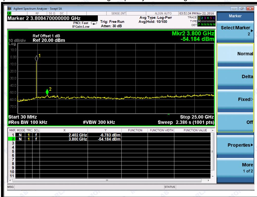
(Plot G.1: Channel = 0, 30MHz to 25GHz @ 8-DPSK)
