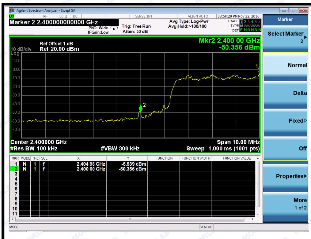
(Channel = 0, Band edge with hopping on @ 8-DPSK)
