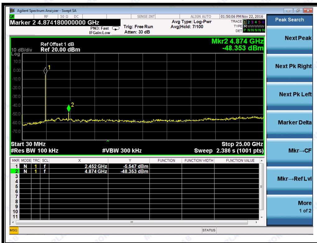
(Plot E.1: Channel = 39, 30MHz to 25GHz @  $\pi/4$ -DQPSK)
