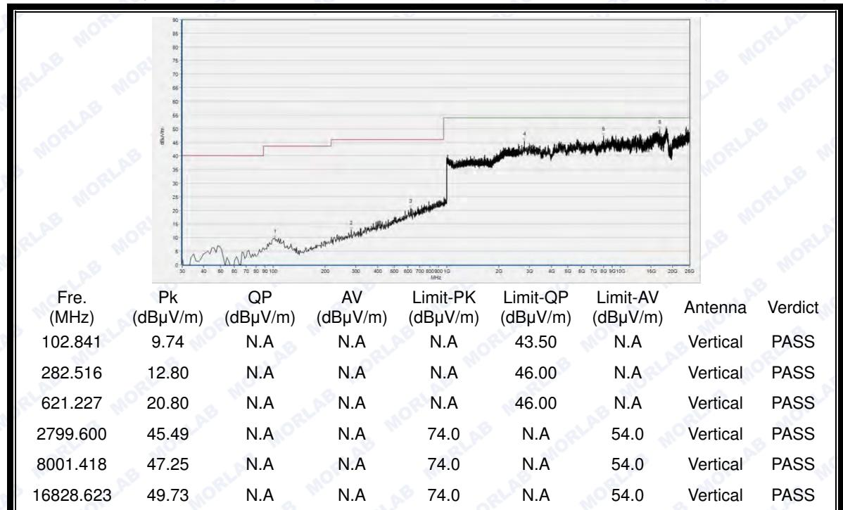
(30MHz to 25GHz, Antenna Vertical @8-DPSK, channel 39)
