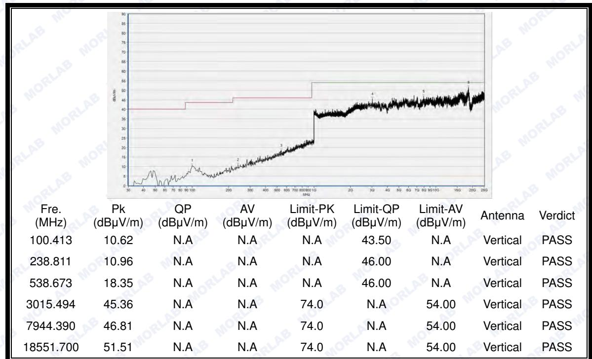
(30MHz to 25GHz, Antenna Vertical @ GFSK, channel 78)
