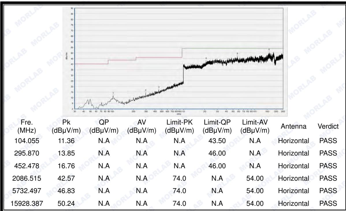
(30MHz to 25GHz, Antenna Horizontal @  $\pi/4$ -DQPSK, channel 78)
