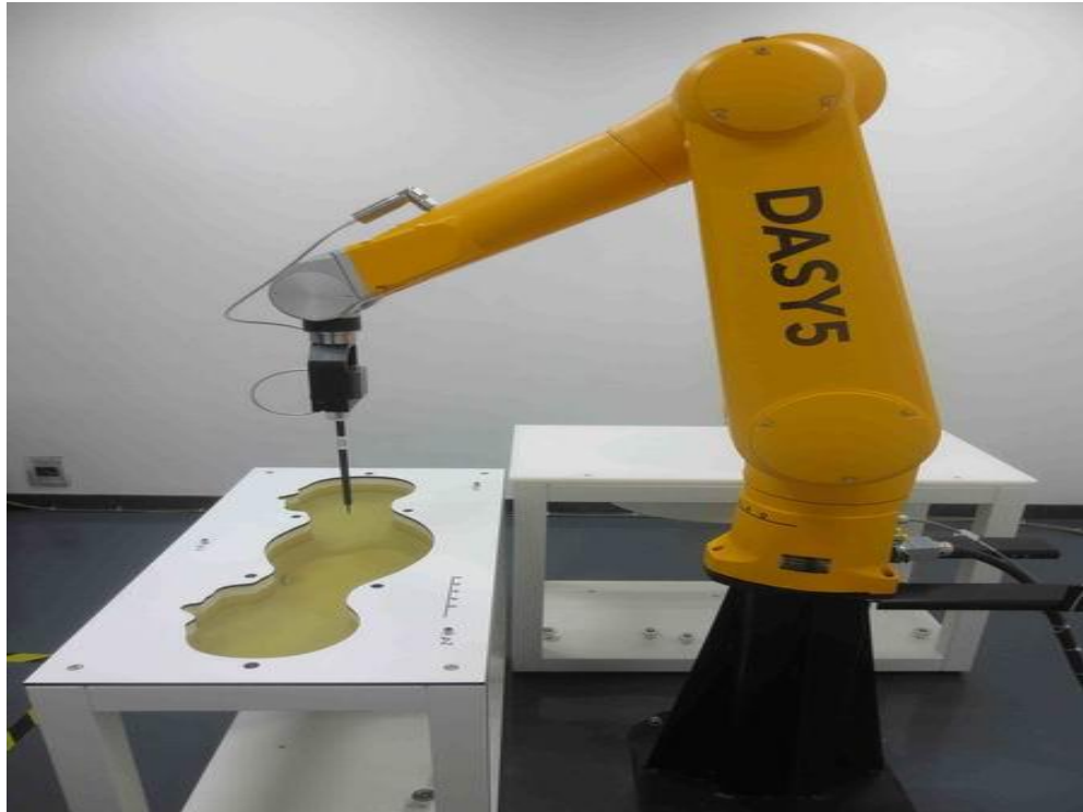
2.4G Liquid depth in the flat Phantom (15cm depth)
