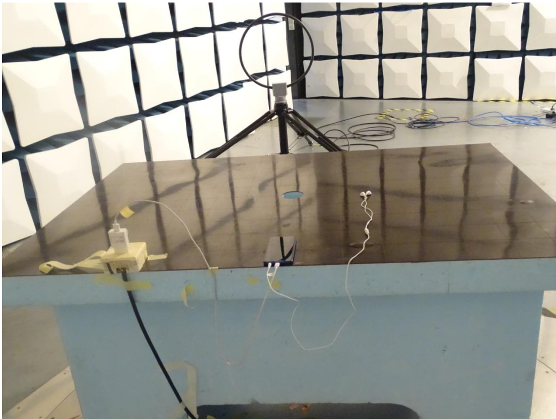
Radiated Spurious Emission (9K-30MHz)
