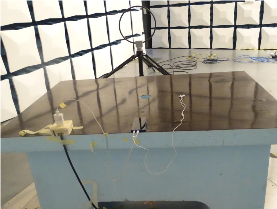
Radiated Spurious Emission (9K-30MHz)
