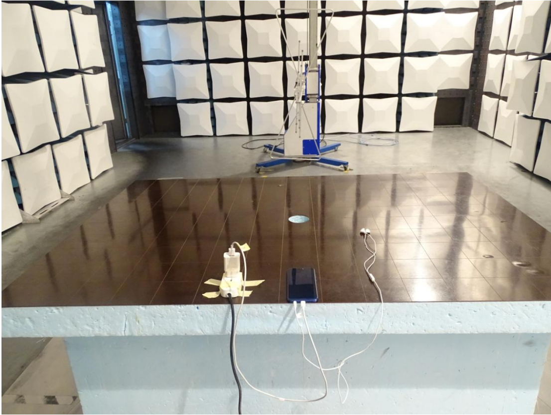
Radiated Spurious Emission (30MHz-1GHz)
