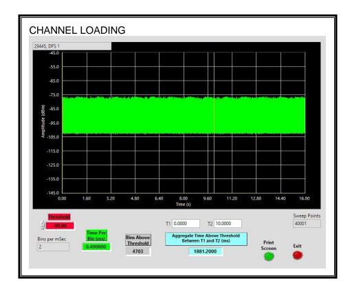
The level of traffic loading on the channel by the EUT is 18.81%.
