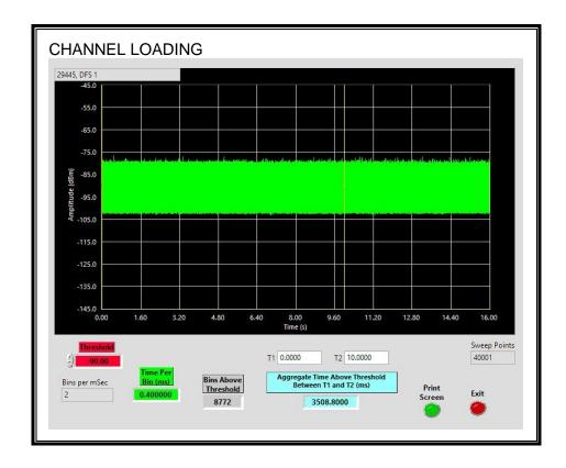
The level of traffic loading on the channel by the EUT is 35.08%
