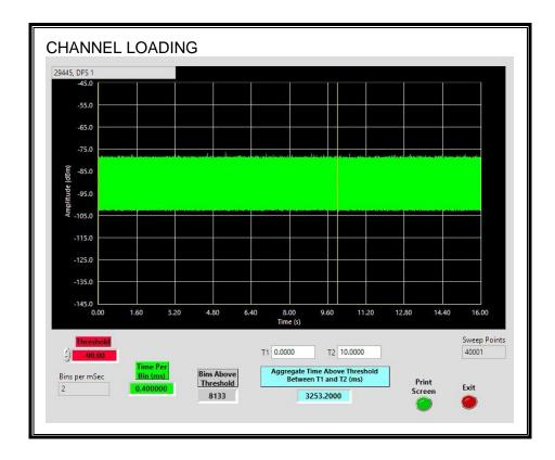
The level of traffic loading on the channel by the EUT is 32.53%.
