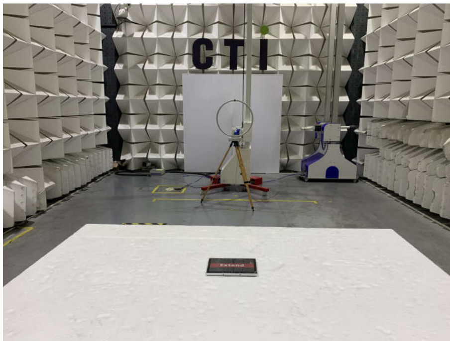
Radiated Spurious Emissions Test Setup (9kHz~30MHz)
