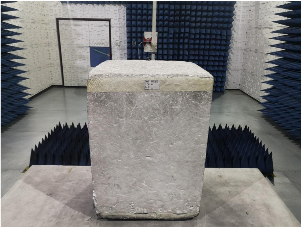
RADIATED EMISSION TEST SETUP ABOVE 1GHz
