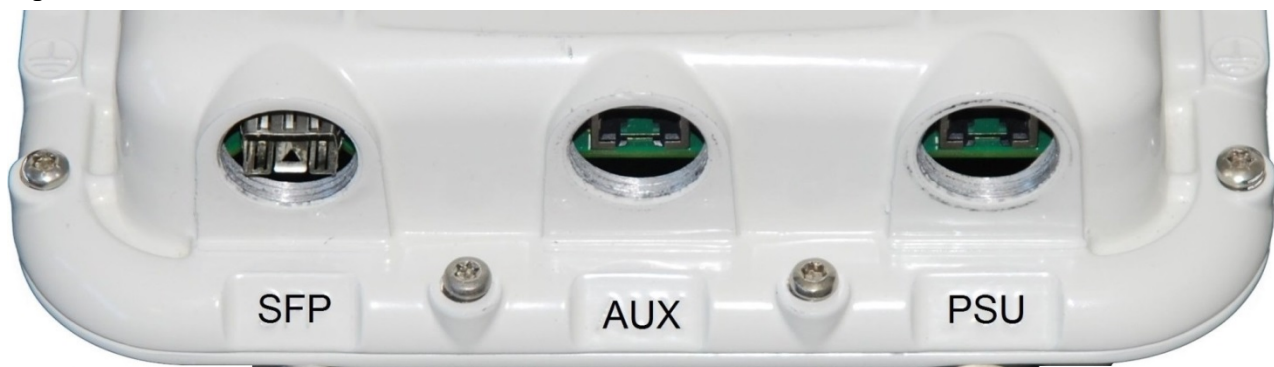
Figure 15 ODU rear interfaces
