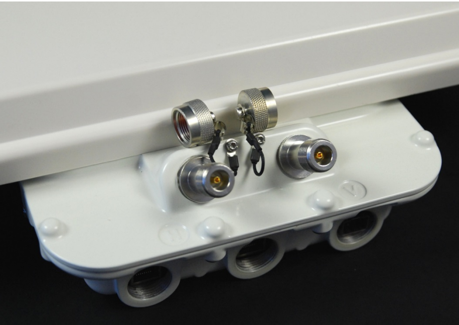
Figure 17 Connectorized+Integrated ODU antenna interfaces
