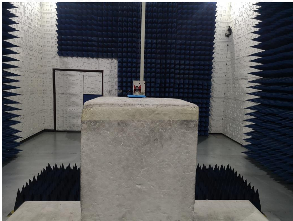
FCC RADIATED EMISSION TEST SETUP ABOVE 1GHZ
