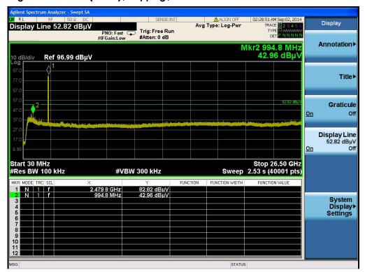
Plot on Configuration For EDR (8DPSK) / Hopping / 30MHz~2400MHz (down 30dBc) (Vertical)
