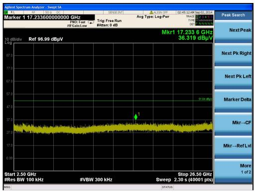
Plot on Configuration For EDR (8DPSK) / Channel 78 / Reference Level
