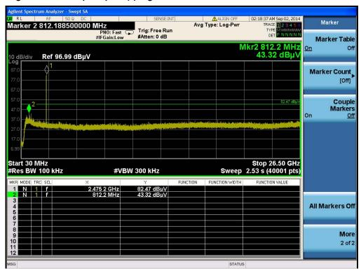
Plot on Configuration For BR (GFSK) / Hopping / 30MHz~2400MHz (down 30dBc) (Vertical)
