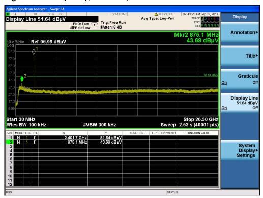
Plot on Configuration For EDR (8DPSK) / Channel 0 / 30MHz~2400MHz (down 30dBc) (Vertical)
