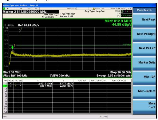
Plot on Configuration For BR (GFSK) / Channel 0 / 30MHz~2400MHz (down 30dBc) (Vertical)
