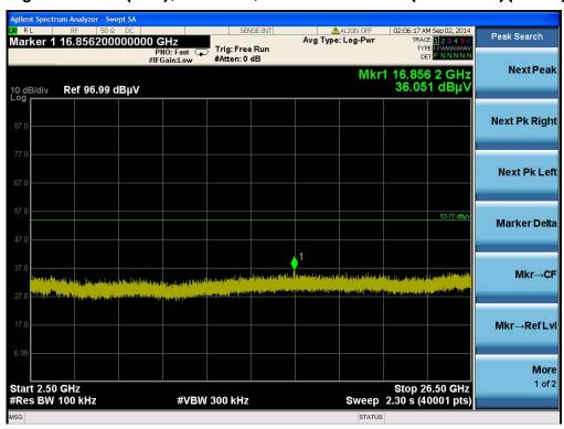
Plot on Configuration For BR (GFSK) / Channel 78 / Reference Level
