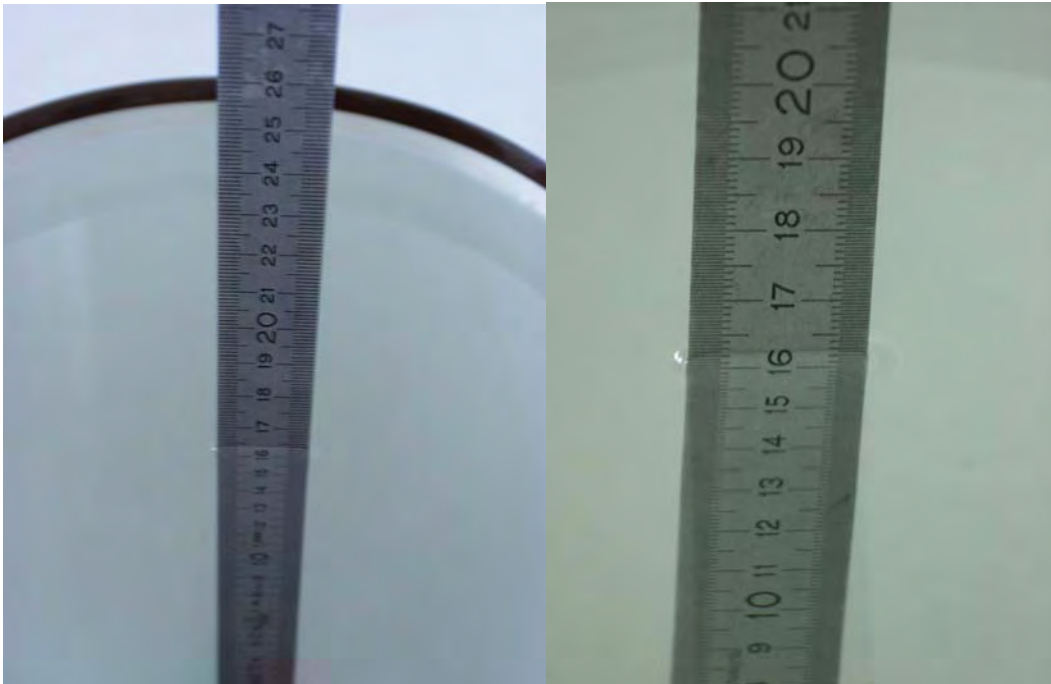
Fig. 36: Liquid depth for PCS 1900 Head and Body measurements.
