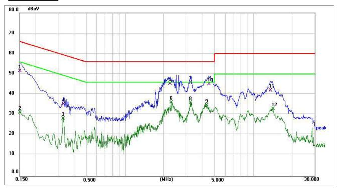
Site: Phase:L1 Temperature(C):23.5(C) Limit: FCC Part 15 C Conduction(QP) **Humidity(%):52.6%**
