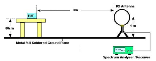
For radiated emissions from 30MHz to 1GHz
