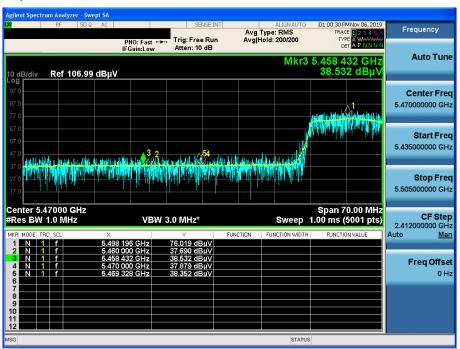
802.11ac(VHT20) & U-NII 2C & Ch.144 & X axis & Ver Detector Mode : AV
