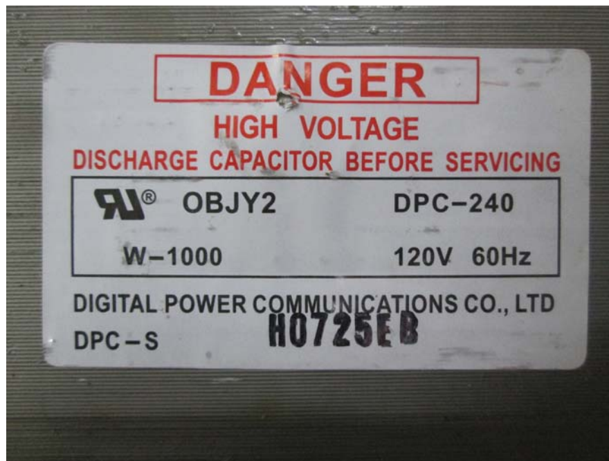
EUT – Transformer Label View
