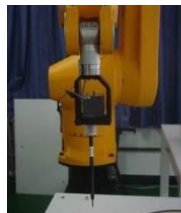
Picture 7-3 E-field Probe
