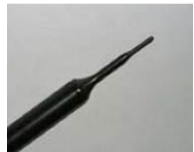
Picture7-2 Near-field Probe
