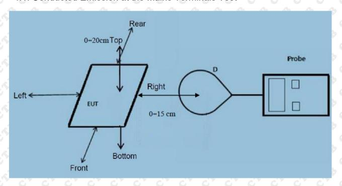
Note: Measurements should be made from all sides and the top of the primary/client pair, with the 20 cm-0cm measured from the center of the top, and 15cm-0cm measured from the center of the rest sides.
