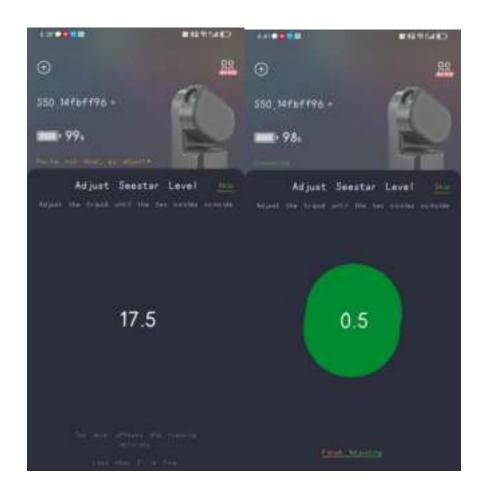
When the device card shows no level, adjust the tripod until the two circles in the picture coincide.
