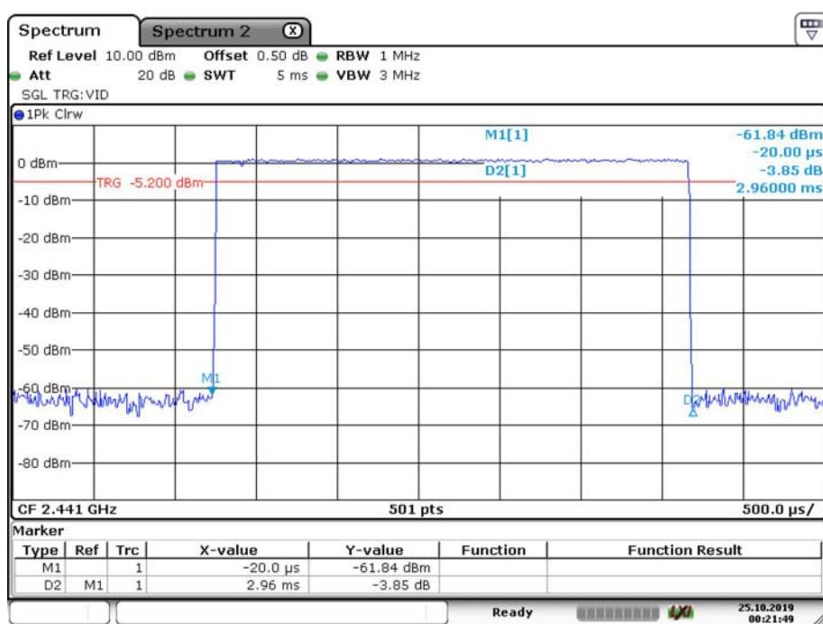
**FCC §15.247(b) (1) - PEAK OUTPUT POWER MEASUREMENT****Applicable Standard**
