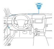
6. Route the wire with USB Type-C plug of the Direct Wire Power Cord to the expected camera mounting location on the windshield.
