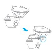
4 Adjust the camera position. There is a mask on the view of the DMS camera. The installer should keep adjusting the camera position to make the driver image fit in the mask. When the mask turned into green, the position of the DMS camera can be regarded as correct.
