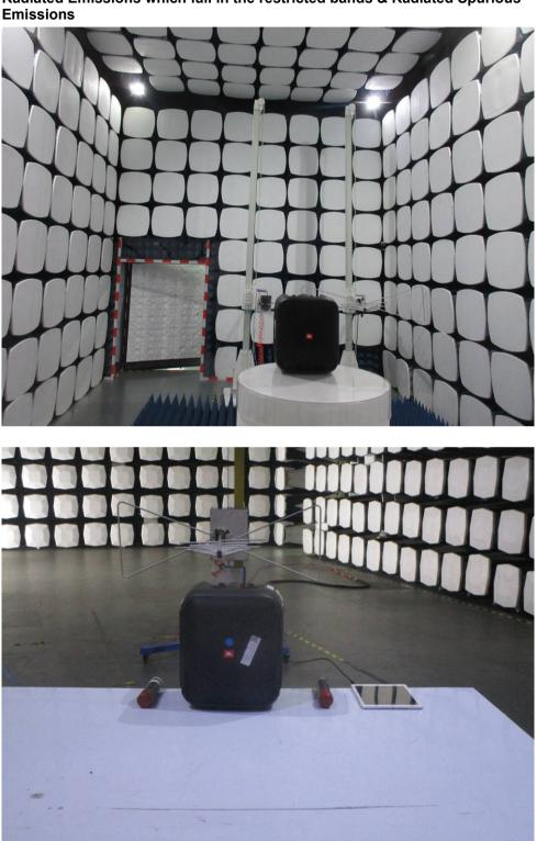
Radiated Emissions which fall in the restricted bands & Radiated Spurious
