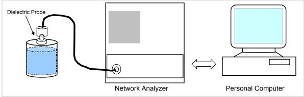
Set-up for liquid parameters check
