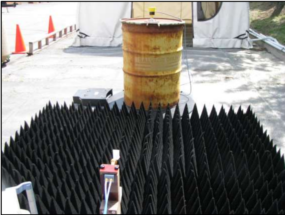
Photograph 8: Radiated Emissions – TC #1; Steel Container, Front View
