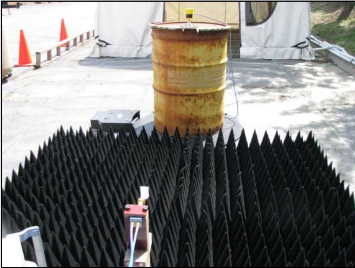
Photograph 12: Radiated Emissions – TC #2; Steel Container, Front View
