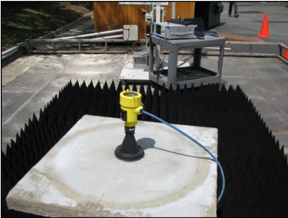
Photograph 10: Radiated Emissions – TC #1; Concrete Container, Front View
