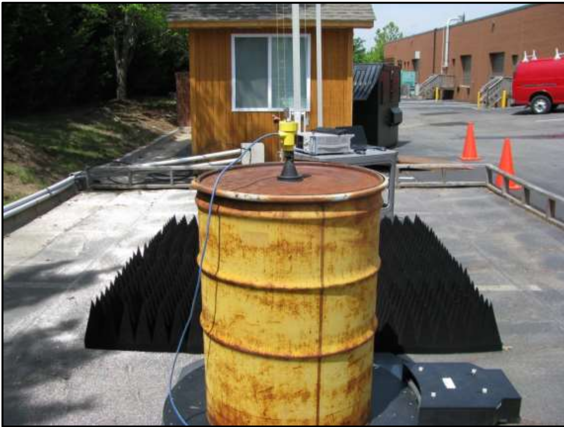
Photograph 9: Radiated Emissions – TC #1; Steel Container, Rear View
