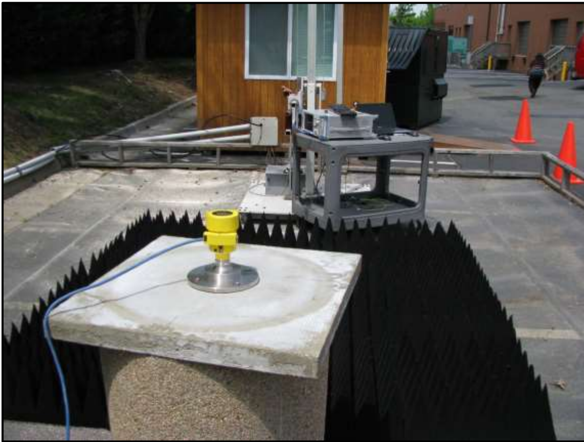
Photograph 14: Radiated Emissions – TC #2; Concrete Container, Front View
