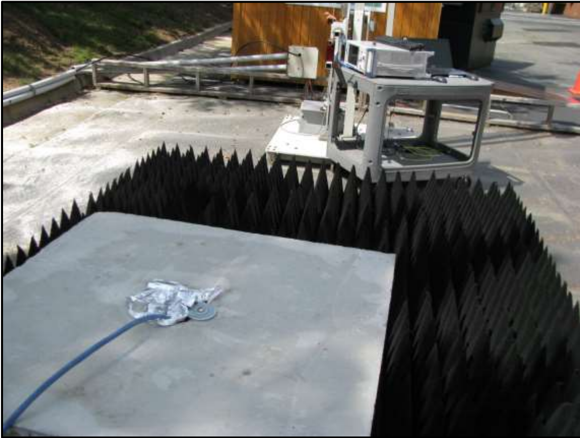
Photograph 23: Radiated Emissions – TC #2 Swivel; Concrete Container, Front View
