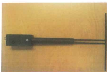
Figure 1 – MVG COMOSAR Validation Dipole
