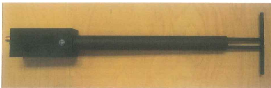
Figure 1 – MVG COMOSAR Validation Dipole
