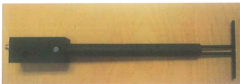
Figure 1 – MVG COMOSAR Validation Dipole
