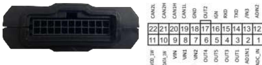
Figure 2. The 22 PIN Connector on the GV350CEU
