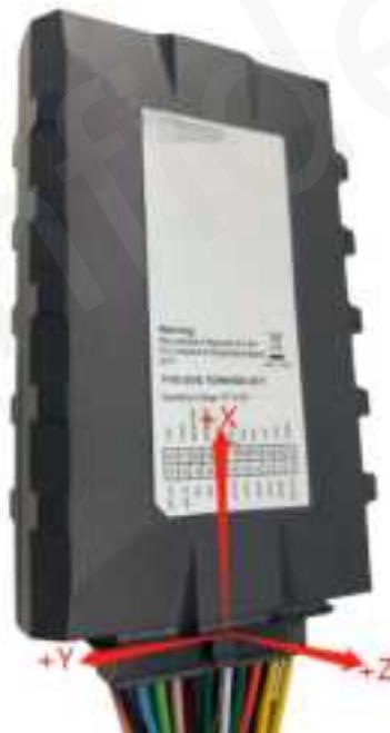
Figure 17. Motion Sensor Direction
