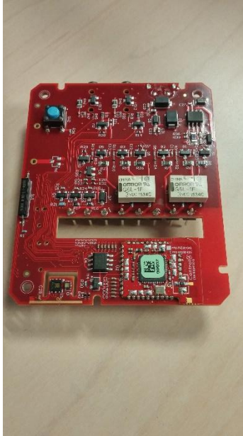
Photograph 1 – Front Side of the C4-Z2IO PCB
