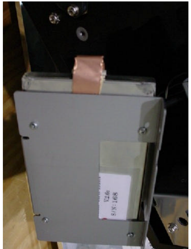
Figure 1.6a Transmitter Ribbon Cable Shielding
