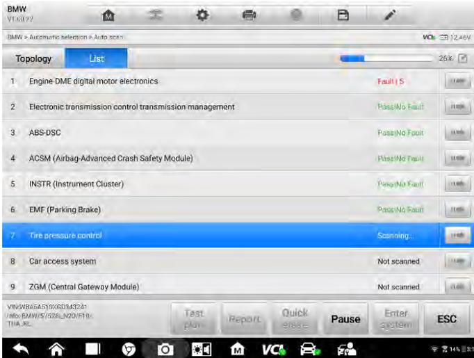
Figure 5-2 DTC Scan
