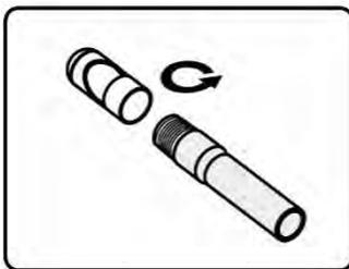
2. Cap and screw the accessory onto the imager head.
