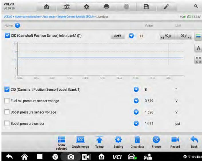
**Figure 4-22 Sample Waveform Graph Mode Screen**
