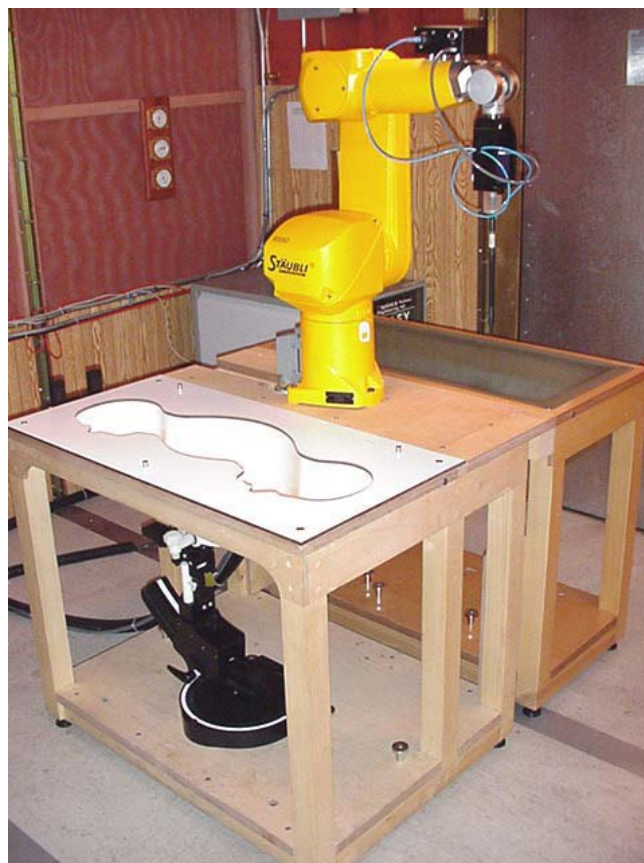
DASY4 SAR Measurement System with SAM phantom
