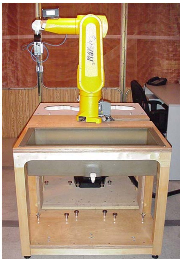
DASY4 SAR Measurement System with Planar phantom
