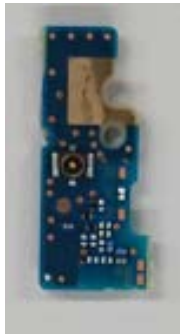
Internal Main_ANT-2-PWB (Front-side)
