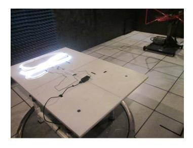
30 MHz - 1000 MHz Radiated Emission 3 Meter OATS
