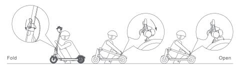
Make sure that the scooter's turned off. To fold, unlock the folding mechanism, and bend the handlebar stem to hook the buckle on the rear mudguard. To open, press the bell trigger to remove from the buckle, erect the handlebar and lock the folding structure.
