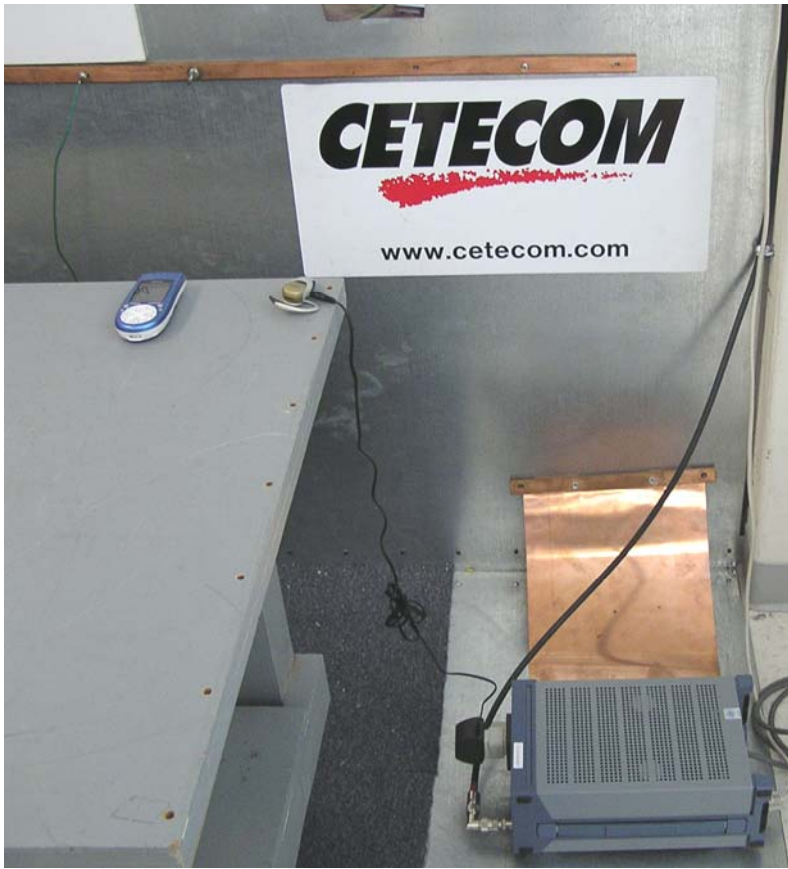
Test setup – AC Line Conducted Emissions
