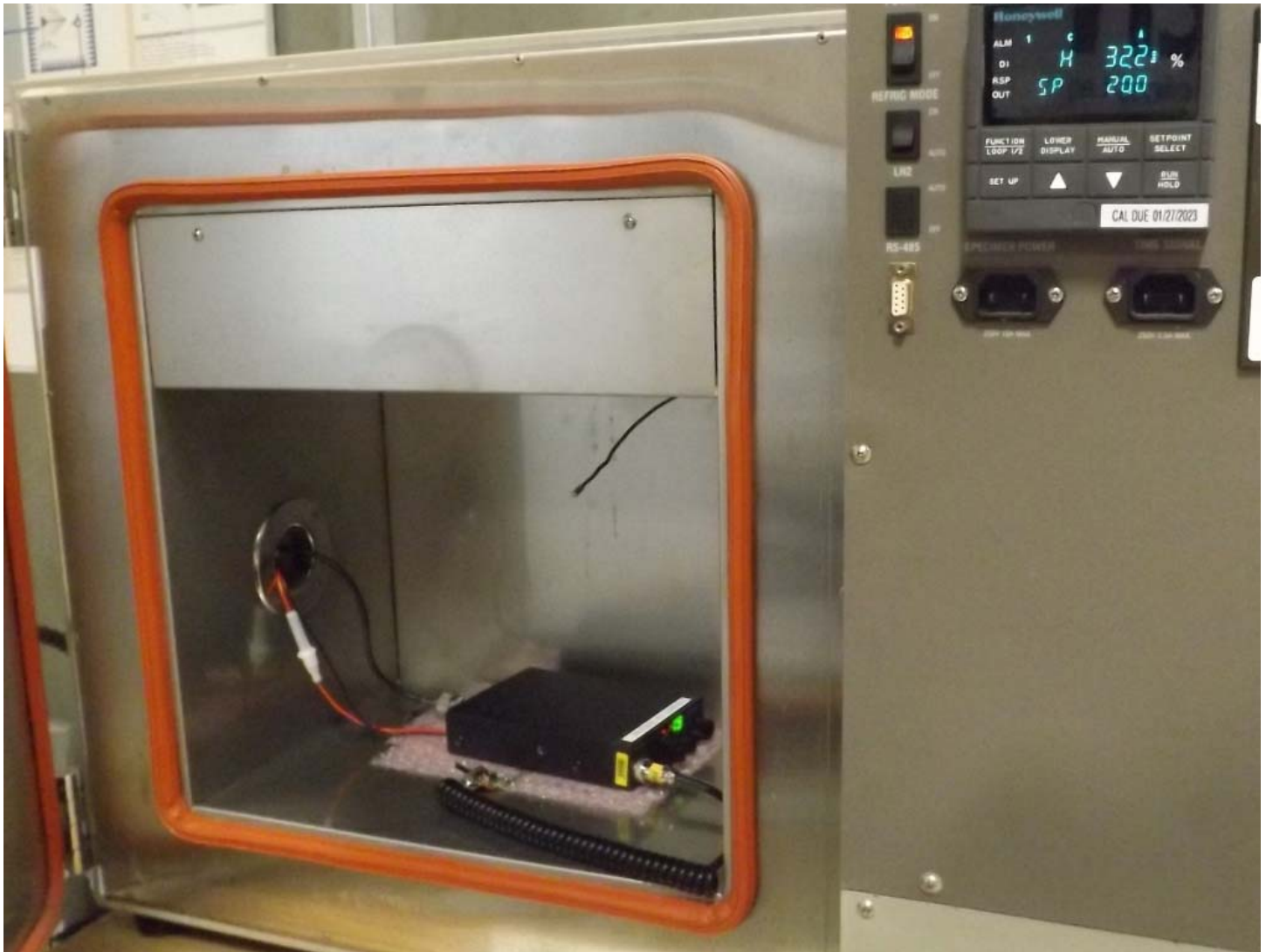
Figure E23.9 – Setup, Frequency Stability
