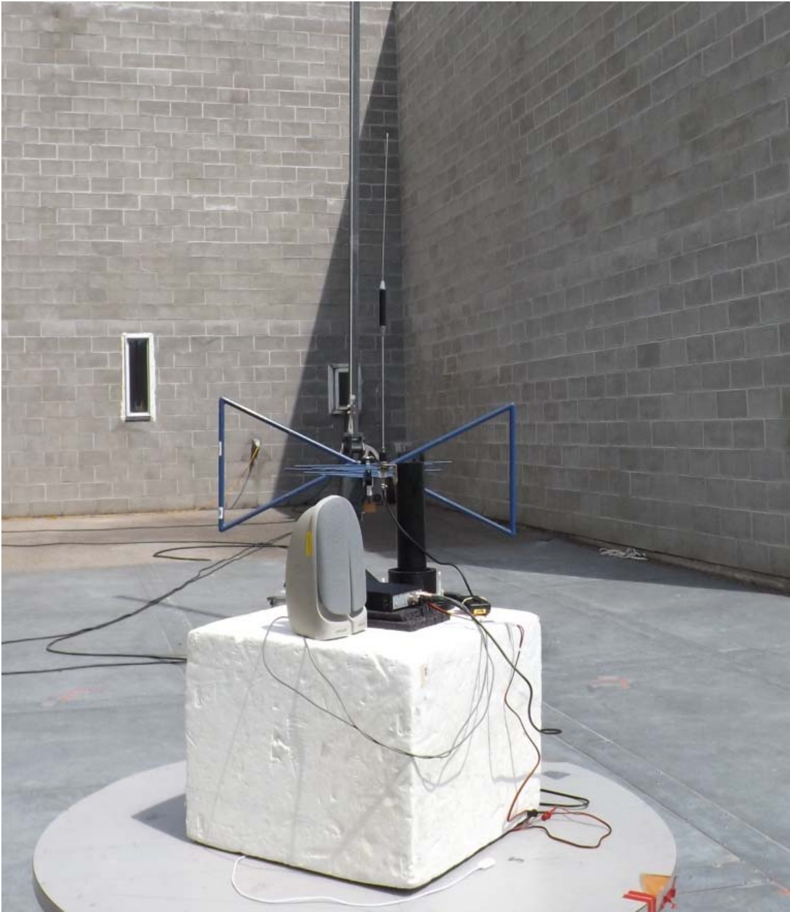
Figure E23.5 – Setup, Radiated Measurements, With Accessories, Horizontal
