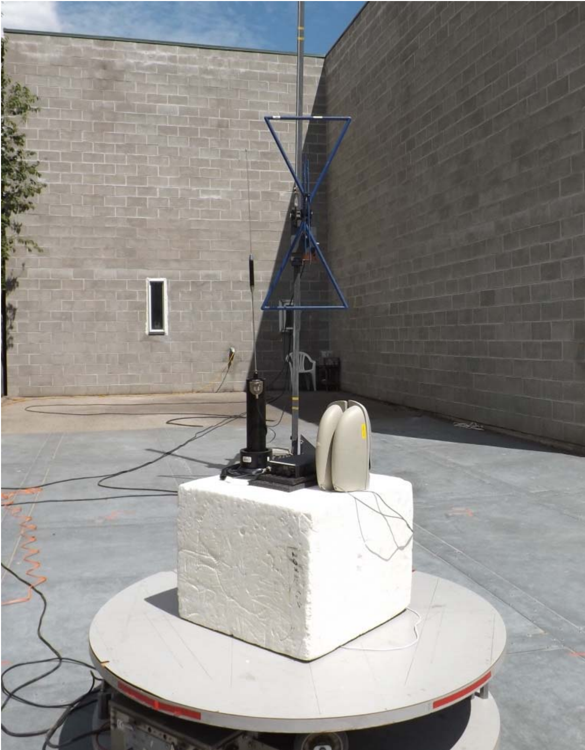
Figure E23.6 – Setup, Radiated Measurements, With Accessories, Vertical
