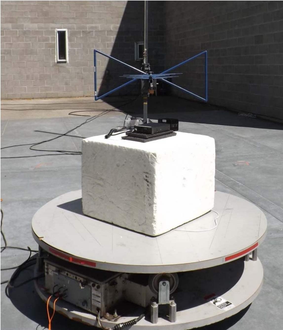
Figure E23.3 – Setup, Radiated Measurements, Without Accessories, Horizontal
