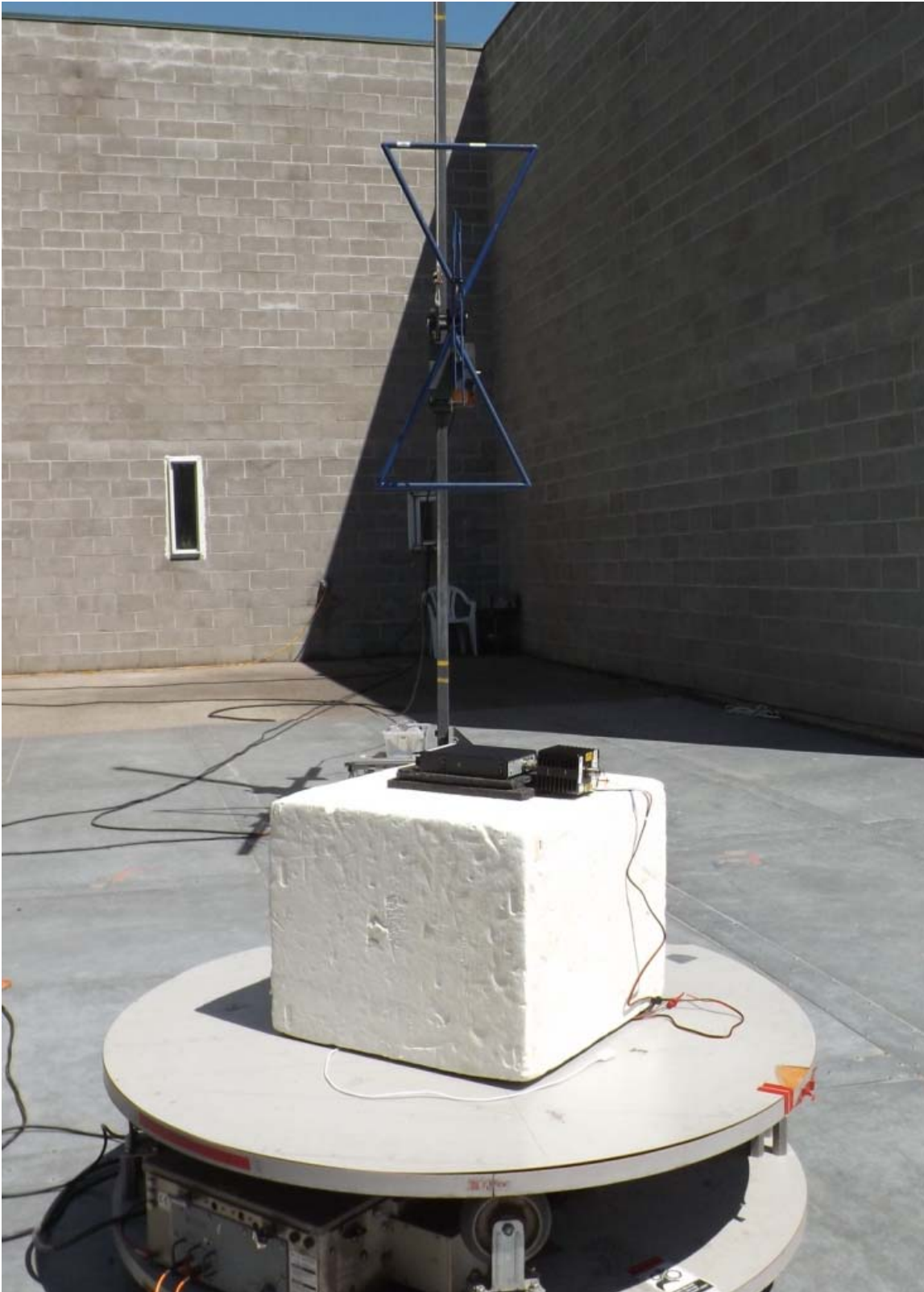
Figure E23.4 – Setup, Radiated Measurements, Without Accessories, Vertical
