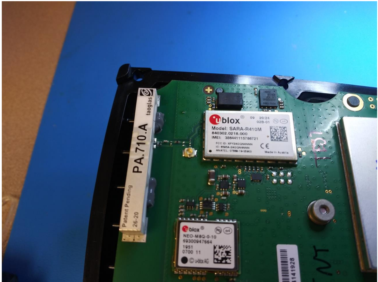
Figure 1 Photograph of UBLOX Module SARA-R410
