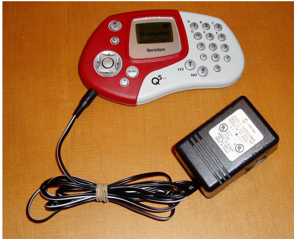
Fig 3 – Front of Q5 RF with 9VDC power supply
