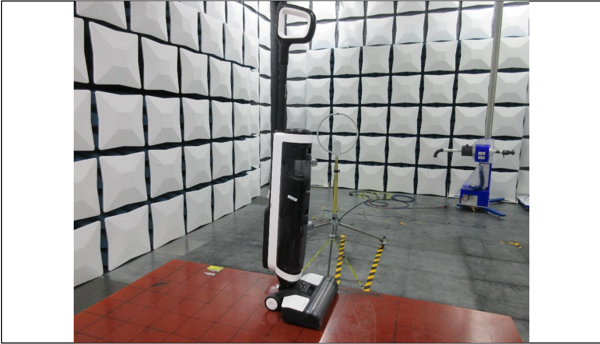
RADIATED RF MEASUREMENT SETUP (Below 30MHz)
