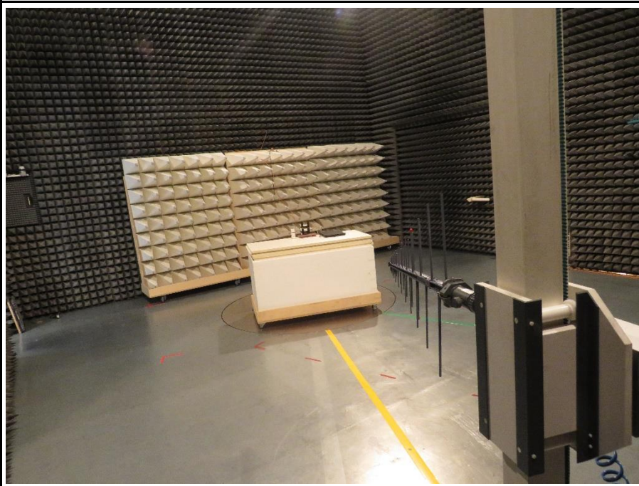
Setup below 1 GHz for Variant 2 (NORA-W101 with external antenna PN PRO-IS-237) -B
